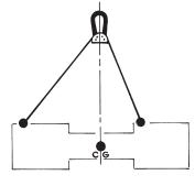
For loads that are balanced and symmetrical, but with lifting points not located in a position for a level lift.
