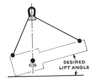
For lifting loads at any desired angle, simply by lifting with sling legs at desired angle.
