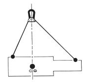
For loads that are heavier on one end, with the center of gravity off-center.
