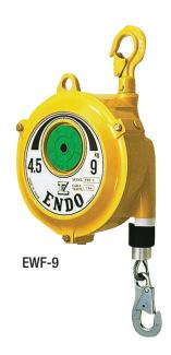
The EWF Series features fully enclosed housing, fall-arrest device (auto-brake), and manual drum locks. If a spring breaks, the brake automatically locks to prevent tool damage. The manual drum lock keeps the drum from rotating to allow easy change out and maintenance of tools. Springs are enclosed in a replaceable cartridge for safe and easy repair.
