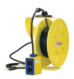
This reel can be used to power moving machinery or used by hand use a customer-installed cable-end accessory. If the accessory weighs over two pounds (0.9 kg), please contact the factory. Reels come with ball stop and various cable types; see Table A on page 9. Three-conductor 110 volt reels come with six foot feeder cord and NEMA 2 molded plug. Four conductor reels are rated NEMA 4 (IP56) for indoor or outdoor use.
