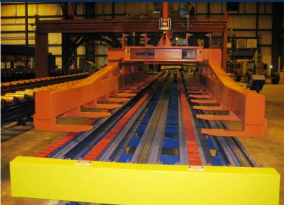
Bushman recently designed this sheet lifter and crane system for a steel and aluminum blanking company. This customer was adding plastic wrapping as a new value-added service. Bushman's heavy duty, motorized sheet lifter picks up 30,000 pound plastic wrapped stacks from a conveyor and puts them on a shipping pallet. This single lifter can safely pick up a wide range of sheet lengths and widths. The lifter has 14 lifting forks on each side, spaced to clear the conveyor rollers, helping to reduce the potential for product damage.
